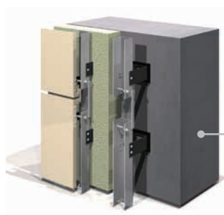
External wall cladding (non-visible hanging cassette system)
