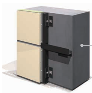
External wall cladding (non-visible cassette system)
