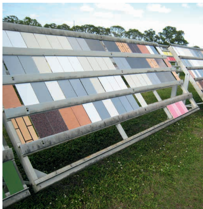
Natural exposure test in Florida, USA
